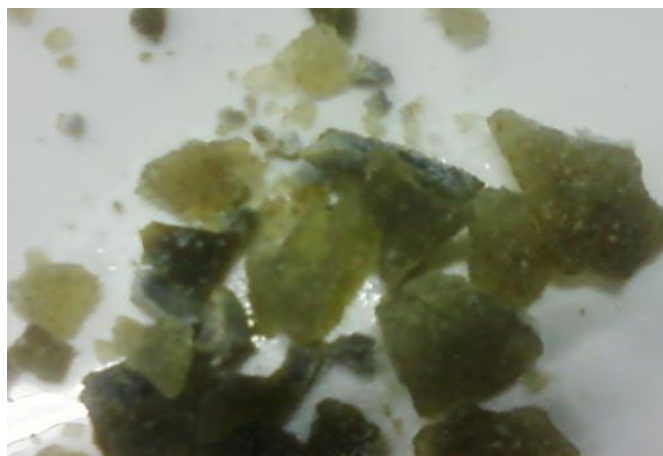
Figure 3. Picture of immobilization of Chlorophyta hydrodictyon africanum in silica gel matrix.
